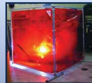
Welding curtains provide a safer work environment, both for welder and those working or walking by the area.
